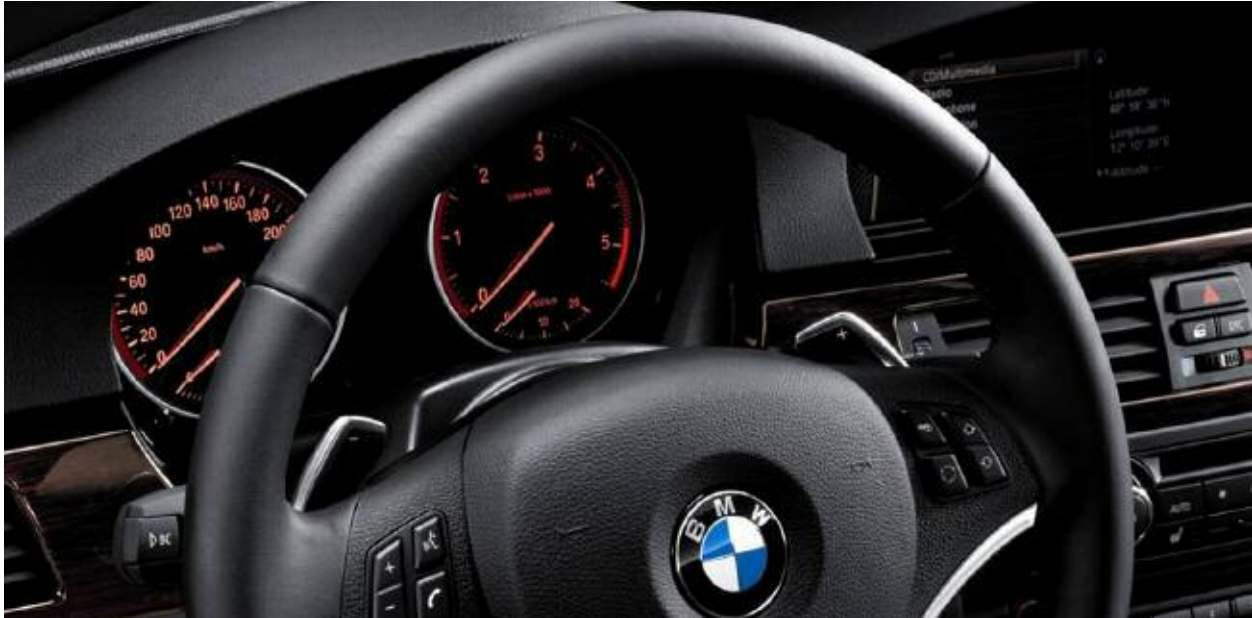
E93/E92 steering wheel with gearshift paddles. Left: Downshift, right: Upshift.
